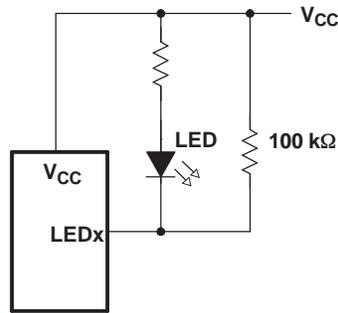
Figure 15. High-Value Resistor in Parallel With the LED
