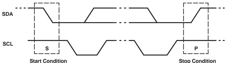
**Figure 1. Definition of Start and Stop Conditions**
