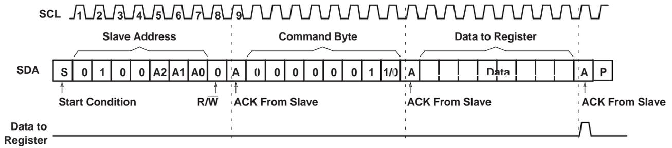
**Figure 7. Write to Configuration or Polarity Inversion Registers**
