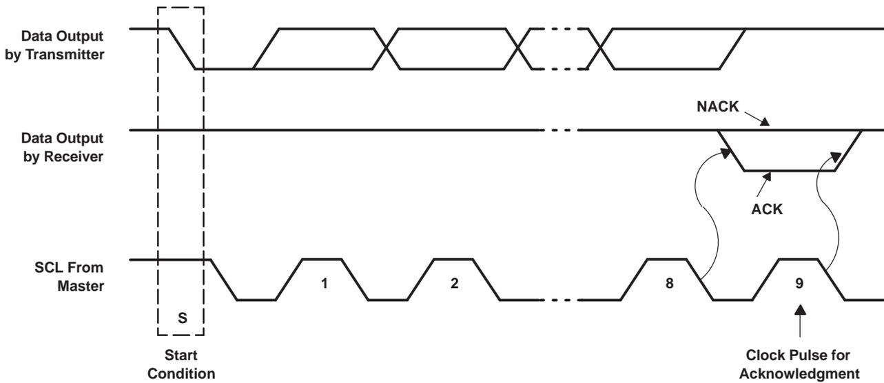
**Figure 3. Acknowledgment on I<sup>2</sup>C Bus**
